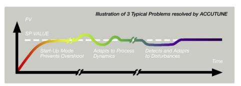
Fuzzy Logic is used to suppress process variable overshoot due to setpoint changes or externally induced process disturbances. It operates independently from Accutune tuning. It does not change PID constants, but temporarily modifies the internal
